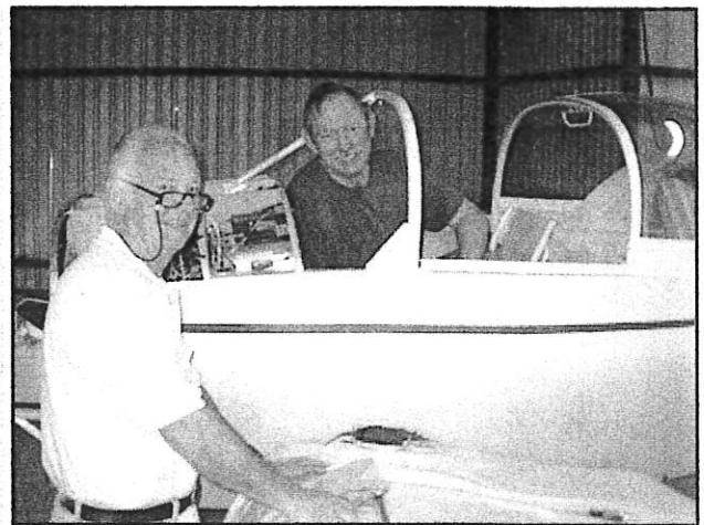
Larry Perryman gets some help on his RV-9A from Ray Coker as they install the bolts in the wing spar for "the last time." Larry will be ready for the Subaru engine package very soon. Looking good!
