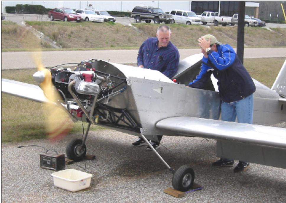
Just before our Feb. 12th meeting, Mike Singleton fired up the VW engine for the first time. (left) It ran fine, but blew the oil cooler due to excessive oil pressure. That has now been corrected.
