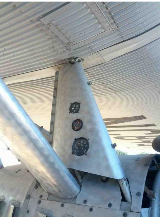
Your left and right engine instruments are outside on the Pylons!
