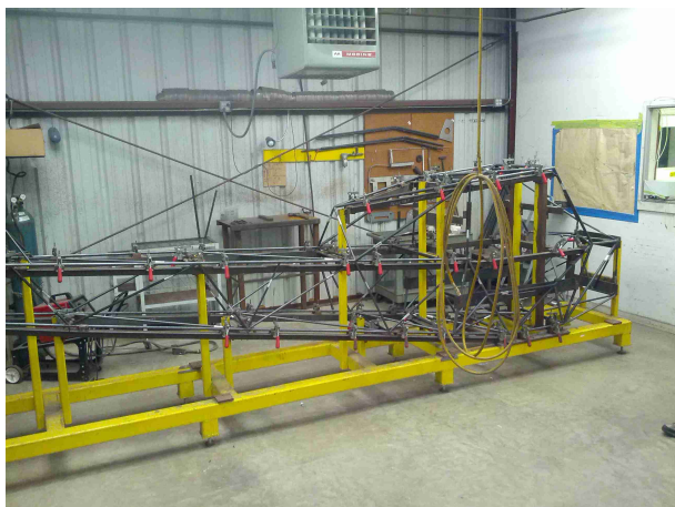
Fuselage tacked in jig
