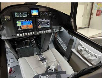
New 302 member Dave Matlock has purchased a near new Van's RV-8 equipped with an IO-390 and constant speed prop. The interior is fully upholstered and the panel sports dual G3-Xs, G-5 and autopilot. Drop by his hanger 44A-2 on the "hill" and check it out.
