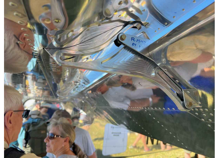
Machined fowler flap tracks
