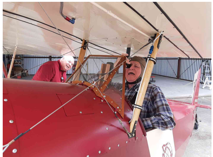
Don demonstrates the periscope he has to use to see the cork float gas gauge on top of the wing
