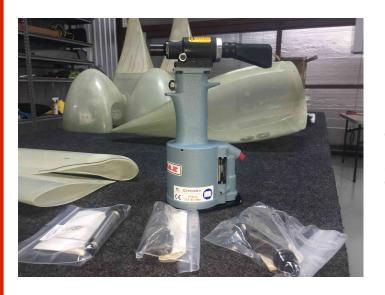
302 member Jose Ruiz, (Joe Cool) has gone out and purchased a new cherry-max rivet puller plus three additional heads for various offsets. This will be available by request from Joe. He lives in Willis 832-515-8108 The gun will pull the much stronger blind rivets that are as strong as a solid rivet.
