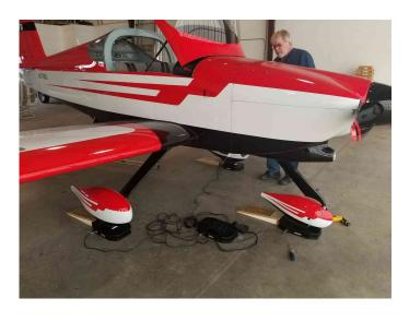
Finally, replaced we have the computer processing unit which came with our aircraft scales. The old one had gone bad, but we were able to find the part instead of replacing the entire \$800 kit. It had to be calibrated, which required a single 550 pound weight. Thanks to Steve Lutte. we located some huge batteries and a certified scale and got the job done.
